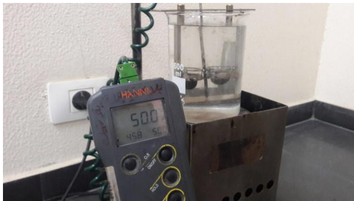
Figure (4.5): Bitumen Samples through the Softening Point Test
