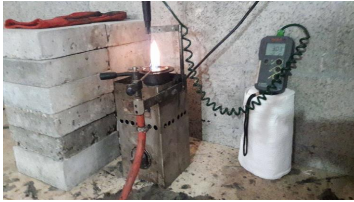
Figure (4.4): Bitumen Samples through the Flash Point Test
