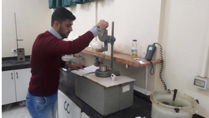
Figure (4.1): Bitumen Samples through the Penetration Test
