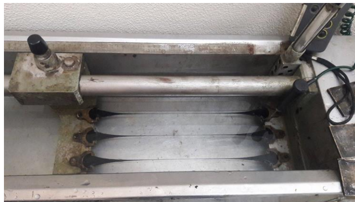
Figure (4.3): Bitumen Samples through the Ductility Test
